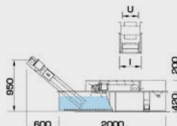
NV7 - NV8 - NV9 Nastro vasca particolari galleggianti e non galleggianti Conveyor with cooling tank for floating and no floating parts
